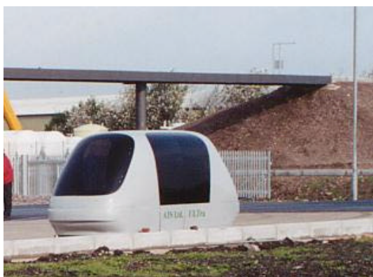
Prototype of the 4-person ULTra PRT vehicle on the test track in Cardiff, Wales, October 2001. The structure in the background is the lightweight bridge for taking the ULTra vehicle over the roadway.
