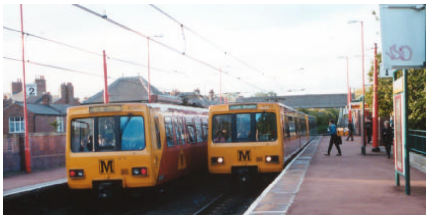
Light Rail Vehicles at Jesmond Station in Newcastle. The Metro system has retained the former heavy rail stations. From March 2002, these vehicles operate over shared track with heavy rail trains along the Metro extension from Pelaw to Sunderland
