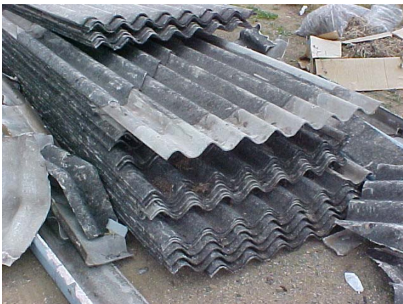
Illegally dumped asbestos (a known carcinogen)
