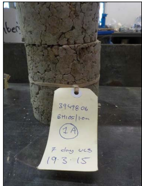
Figure 10: Bore 105/1.0 m 3% Lime – Sample 1A (un-soaked prior to testing)
