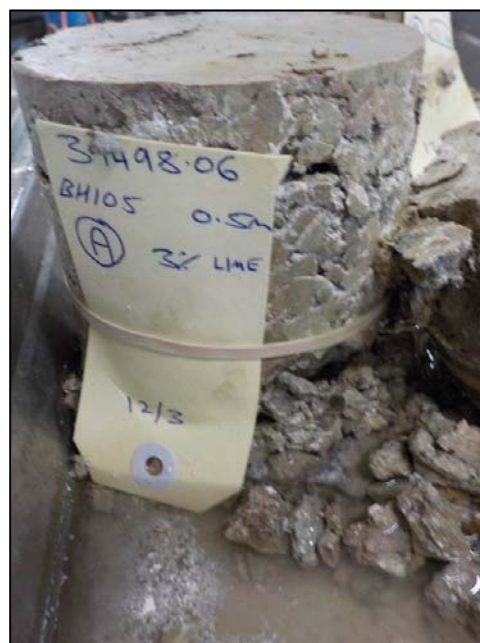
Figure 6: Bore 105/0.5 m 3% Lime – Sample A
