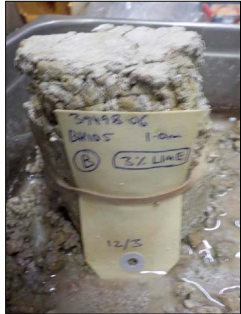
Figure 8: Bore 105/1.0 m 3% Lime – Sample B
