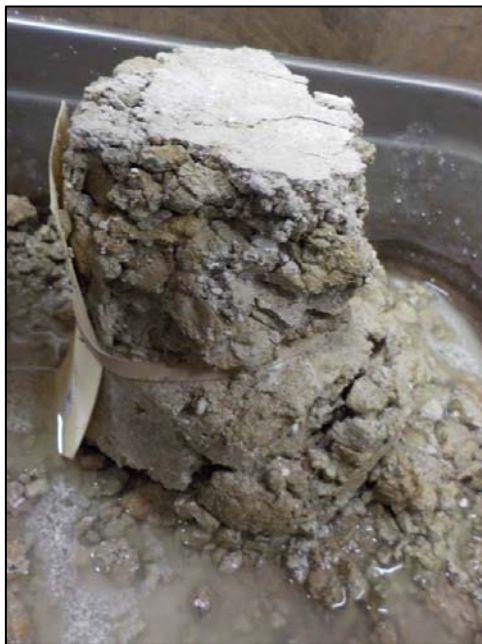
Figure 9: Bore 105/1.0 m 3% Lime – Sample B
