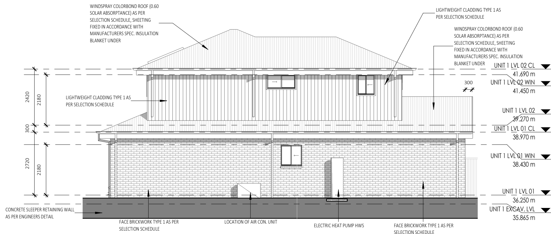
WEST ELEVATION - UNIT 1 1 : 100
