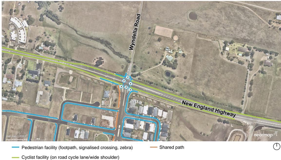
Figure 2-5 Walking and cycling infrastructure – Wyndella Road/ New England Highway
