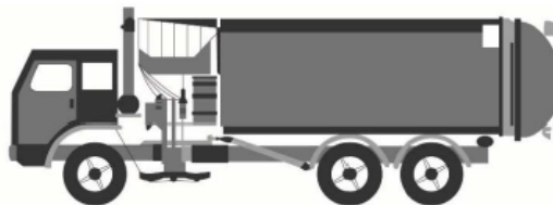
Side-loading waste collection vehicle
