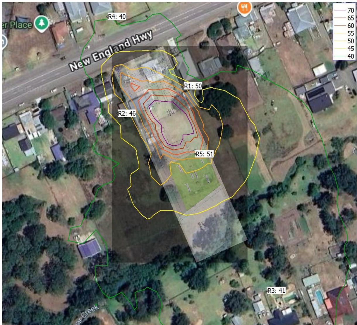
Figure 4-1 Cumulative Operational Results dB(A) Leq(15min)
