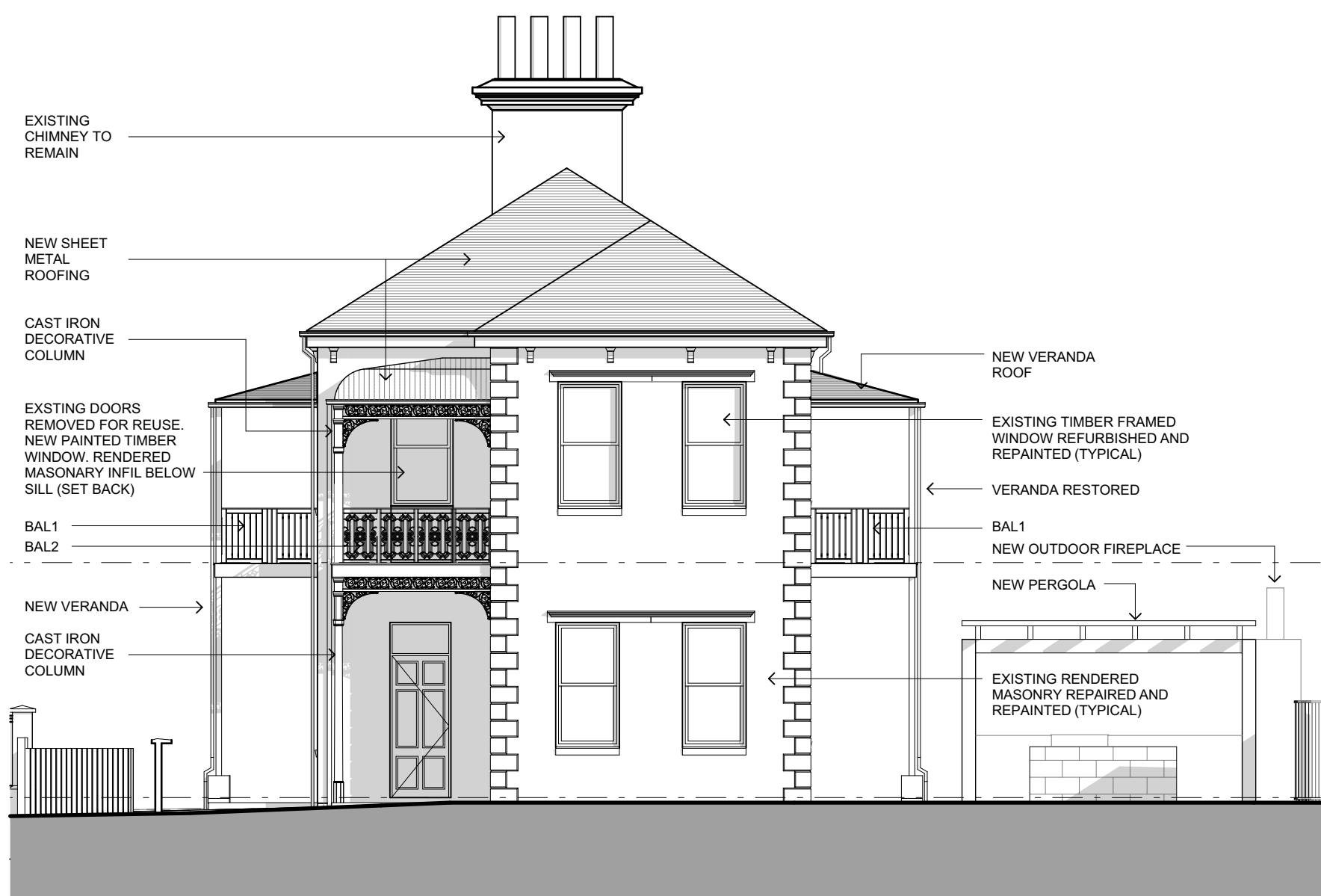
House - East Elevation 1:100
