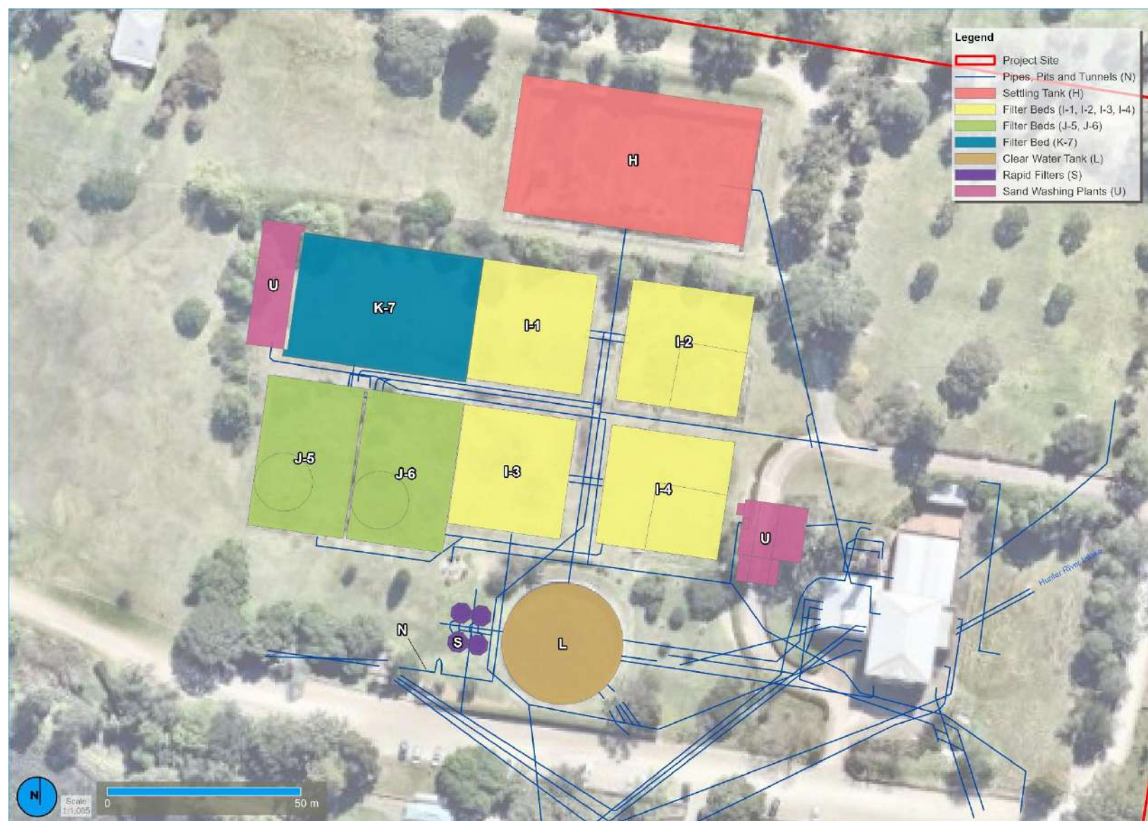
Figure 94: Main elements of the filtration system. Note the pipe network extends to the reservoir to the south, and beyond the Project Site Boundary to the east.
