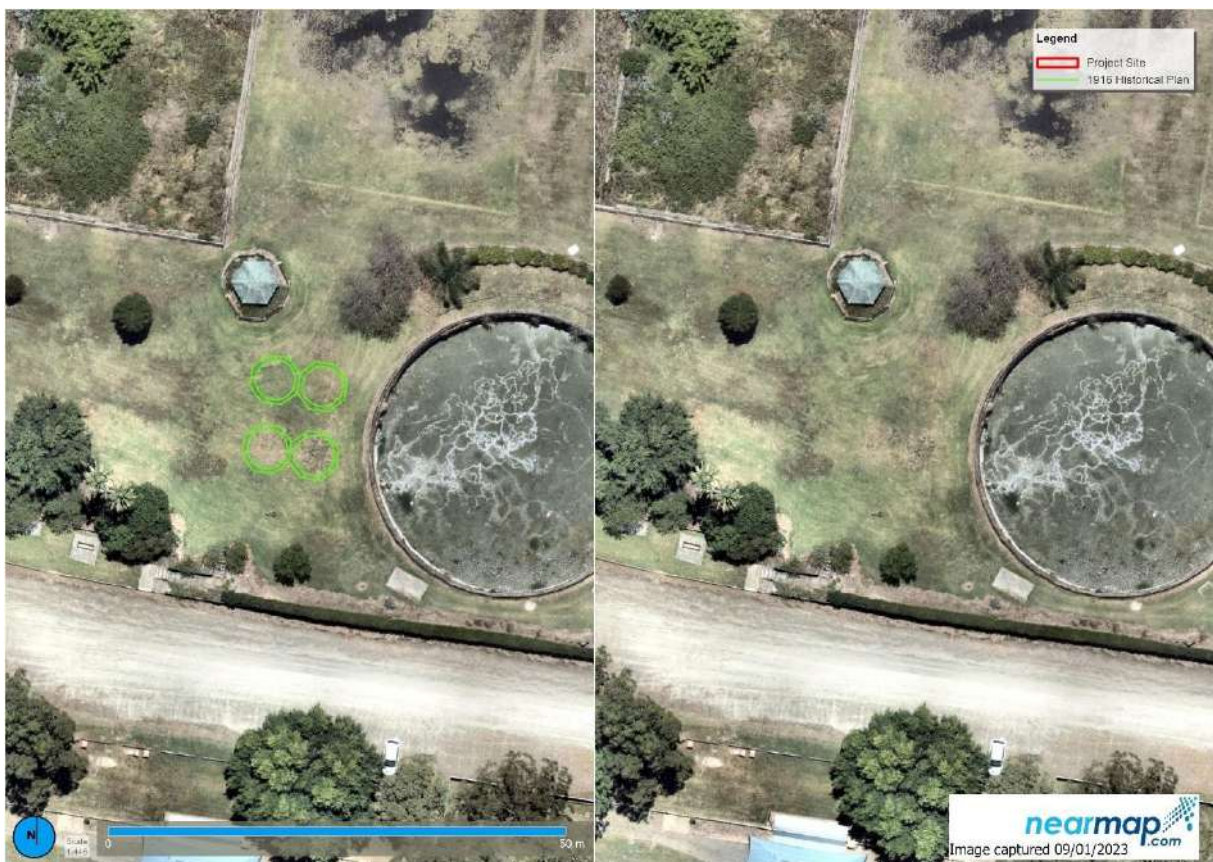
Figure 123: Analysis of the 2023 aerial photo of the site where the four Rapid Filters can be discerned as patches of drier grass.
