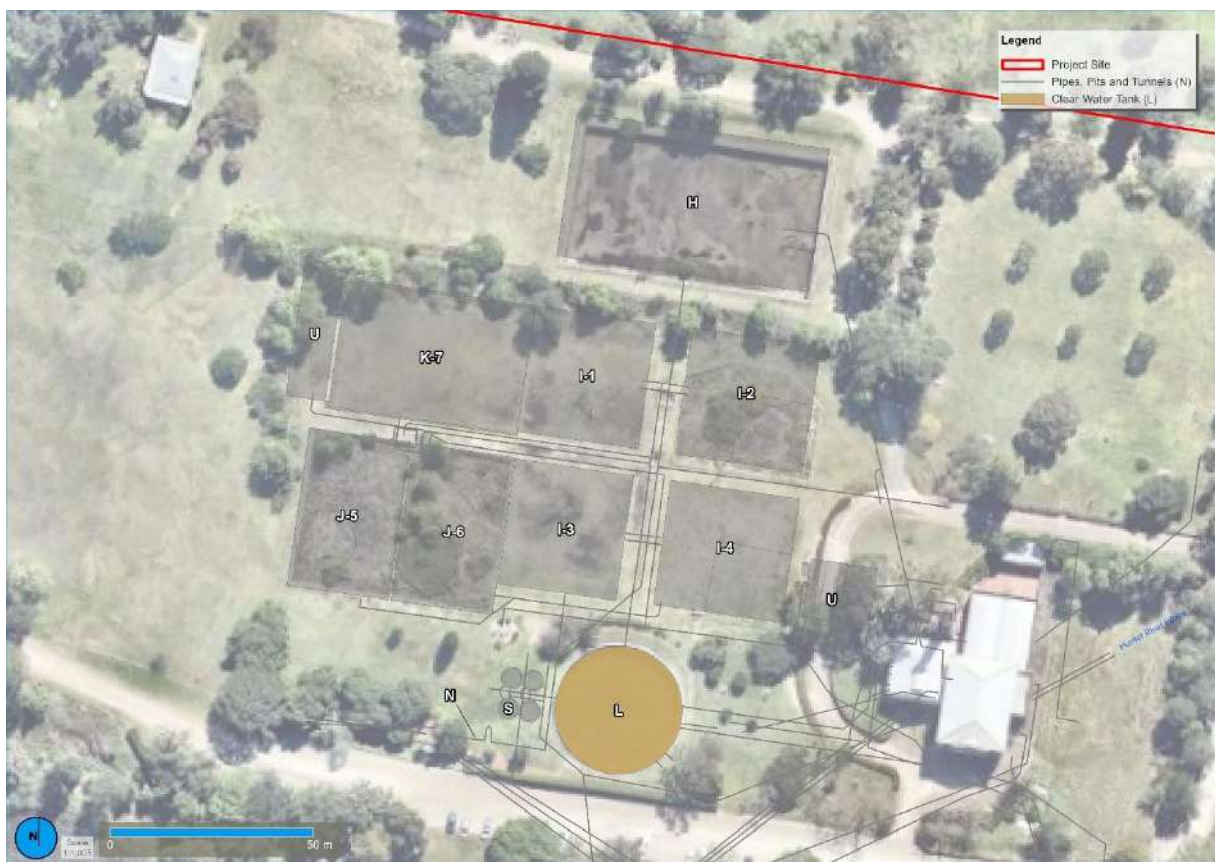
Figure 110: Location of the Clear Water Tank and the southern end of the Filtration System
