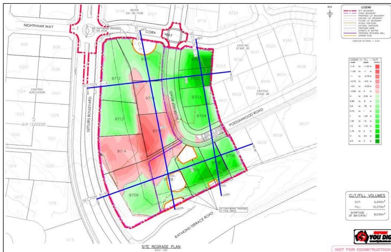
Figure 6: Site Regrade Plan Source: ADW Johnson (April 2026)
