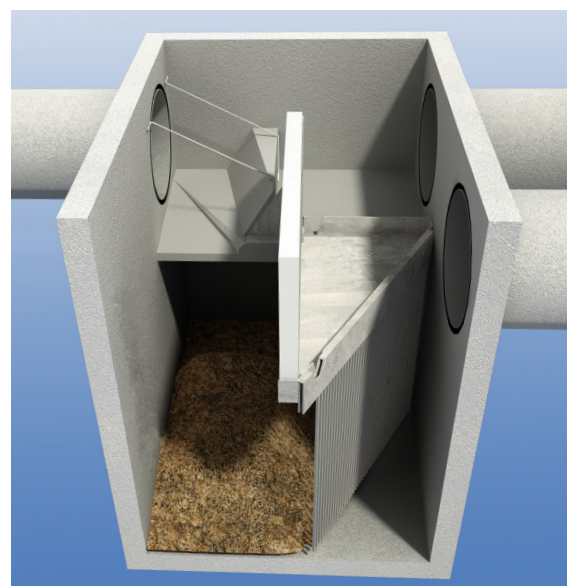
Figure 4 – Dual Outlet HumeGard® GPT
