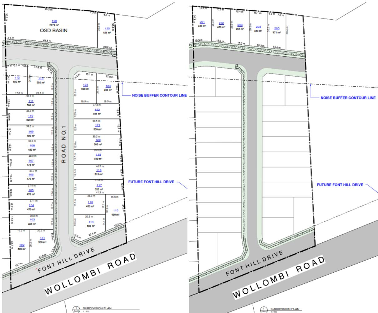
**Figure 5:** Staged subdivision plans, Stage 1 left above, Stage 2 right above (Prepared by the Bathla Group)
